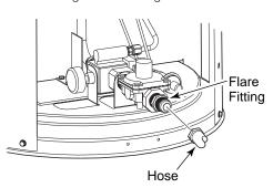
Figure 3 - Hose and Valve Inlet
